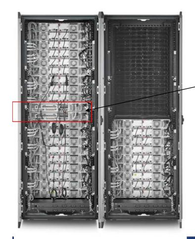
EE Array directly connects to the system switch or controller
