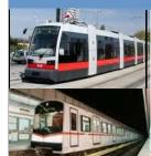
Metro: 94,7 % recyling components/materials 30 % less energy use as the last model. 44 Metro trains / Metro-control technology, energy supply ULF: 300 ULF- ultra low floor light rail trams Energy saving 30 % through regenerativ braking 2012 -2020: + 150 ULF + 4 Metros p.a. + control technology + 12 ebuses (2012) + eticketing (2014) Extension U1 (2015), U2 (2013 Seacity Aspern)
